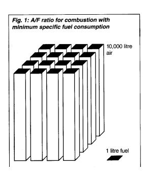
Spark-ignition engines achieve their maximum output at air-deficiency levels of 5...15% ( $\lambda = 0.95...0.85$ ), while minimum fuel consumption is achieved with an air excess of 10...20% ( $\lambda = 1.1...1.2$ ).  $\lambda = 1$  provides optimum idling characteristics.
