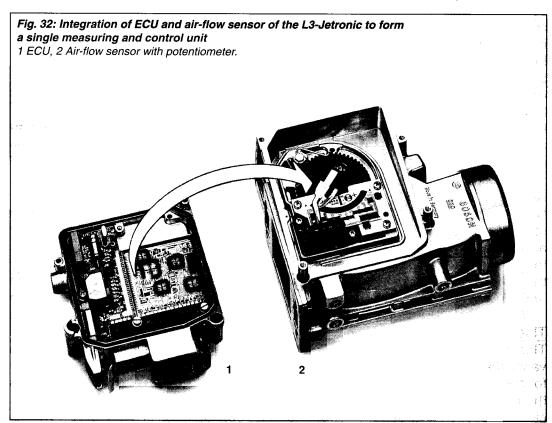
intake-manifold pressure is maintained constant at 2.5 or 3 bar so that the quantity of fuel injected depends solely upon the opening time of the injection valves. For this purpose, the control unit supplies control pulses, the duration of which depends upon the inducted air quantity, the engine speed and other actuating variables which are detected by sensors and processed in the control unit.
