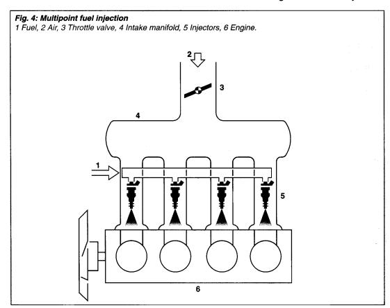
filling (volumetric efficiency) and higher torque. The results are enhanced specific output and an improved torque curve. Mono-Jetronic also conforms with standard practice in incorporating separate arrangements for measuring air and metering fuel; the reduction in the length of the throttled section of the intact tract also provides higher outputs (compared with the carburetor).
