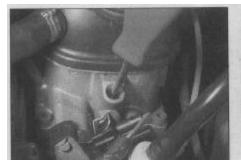
10.3a Idle speed adjustment screw location
