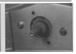
15.3a Bolts securing the window regulator to the door
