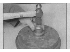
10.9 Drive the outer races securely into position using a socket on the outer edge
