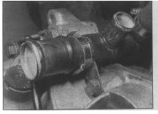
2.8 Coolant pipe support bracket location
