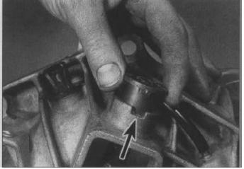
5.9 Showing the location tab (arrowed) on the release shaft outer bush
