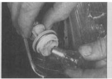
5.14c . . . and remove the front direction indicator bulb
