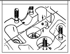
4.22b Minimum distance (a) between top of valve guides and upper surface of cylinder head
