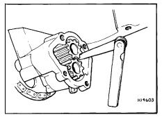
14.10 Checking the oil pump gear backlash
