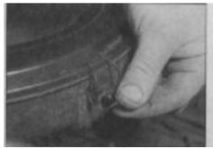
17.1a Unclipping the air cleaner top cover - single-point fuel-injected models
