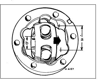
4.22 Assembly of the inner joint cage and hub to the housing
