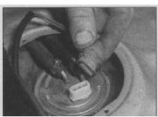
7.8 Unplug the wiring harness connector from the pump/sender unit
