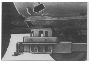
Workshop hoist/trolley jacking point for the front of the vehicle
