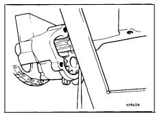
14.11 Checking the oil pump gear axial clearance
