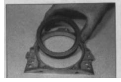
8.14 Removing the seal from its housing
