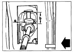
4.8 Gear lever adjustment dimensions a 11.0 mm b 43.0 mm
