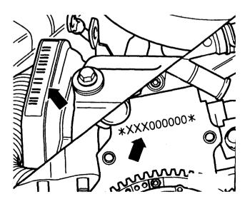
Engine number and engine code locations (arrowed)
