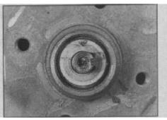
10.4a Rear wheel bearing thrustwasher
