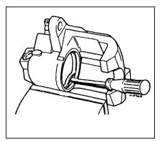
8.8 Extracting the piston seal - take care not to scratch the surface of the bore
