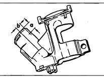
16.9 Drill a 3 mm hole at the point shown to reveal the lock cylinder detent plunger
