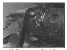
9.7a Starter motor retaining bolts, showing exhaust bracket location
