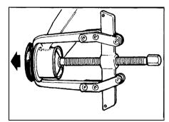
12.5 Use a puller to remove the rear axle beam pivot bushes
