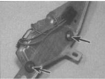
13.4 Tailgate wiper motor mounting bolts on the bracket
