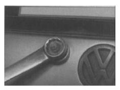
13.2a Unscrew the tailgate wiper motor outer nut . . .
