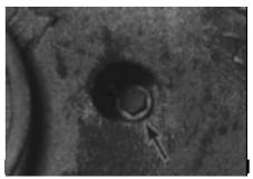
15.4 Remove the plug in the inner wheel arch to gain access to the crankshaft pulley bolt (arrowed)
