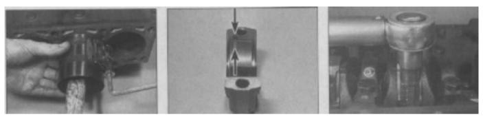
12.16 Using a piston ring compressor to install the piston assemblies
