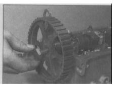
4.71 Refitting the camshaft sprocket and bolt
