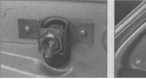
20.6 Exterior mirror control locknut and control knob on the inside of the door
