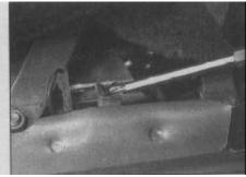
19.3 Unscrewing the handbrake warning light switch mounting screw
