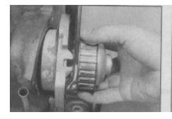
7.6a Removing the water pump
