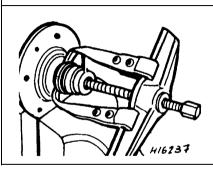
5.4 Using a puller to remove the outer wheel bearing race from the hub
