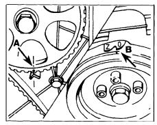
2.16 Camshaft sprocket (A) and crankshaft pulley (B) timing marks
