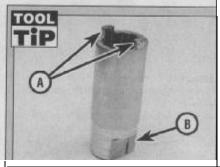
In the absence of the special VW tool, a replacement can be fabricated from a long-reach 13 mm socket. Cut the lower end of the socket to leave two teeth (A) which will engage with the slots in the strut nut, and file the upper end of the socket (B) so that it can be held with an open-ended spanner
