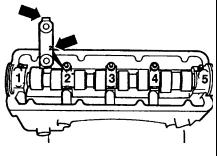
4.64 Camshaft bearing cap markings and orientation
