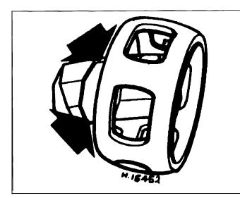
4.17b Removing the inner joint hub from the cage
