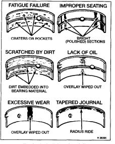
8.8 Typical shell bearing failures
