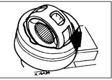
4.7 Removing the cage and hub from the outer joint housing Arrow shows rectangular aperture
