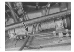
17.5 Clutch cable hole (arrowed) in the steering gear housing
