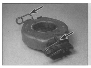
5.3 Release bearing showing retaining clips (arrowed)
