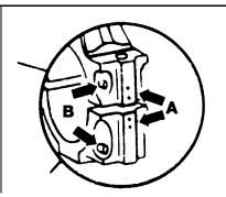
5.20a Big end bearing cap and connecting rod markings A identification (cylinder number) markings B Orientation recesses
