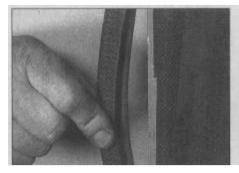
25.8 Pull away the weatherstrip before removing the rear trim panel
