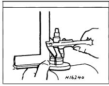
9.3 Checking the rear wheel stub axle for distortion
