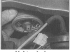
5.3 Disconnecting the wiring plug from the rear of the headlamp bulb
