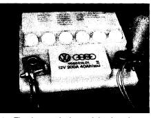
1 The battery is located in the plenum chamber at the rear right-hand side of the engine compartment. The exterior of the battery should be inspected periodically for damage such as a cracked case or cover.
