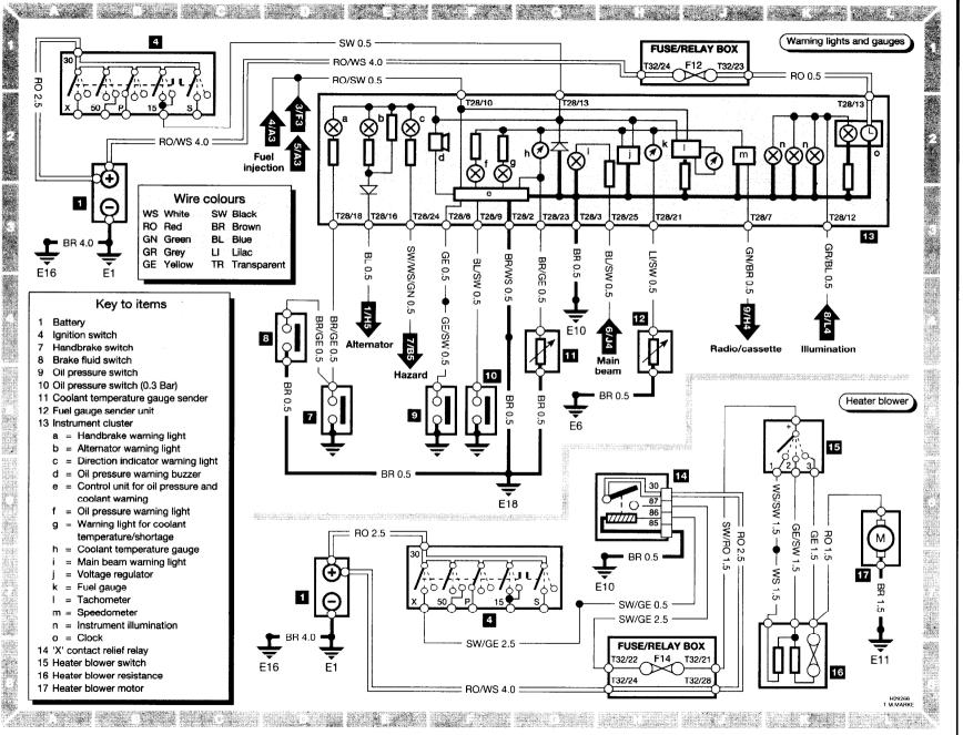
Diagram 2 : Warning lights, gauges and heater blower
