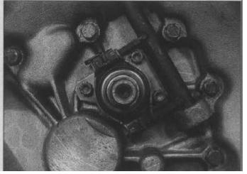
5.2 Release bearing in place on the release shaft arms (four speed transmission)
