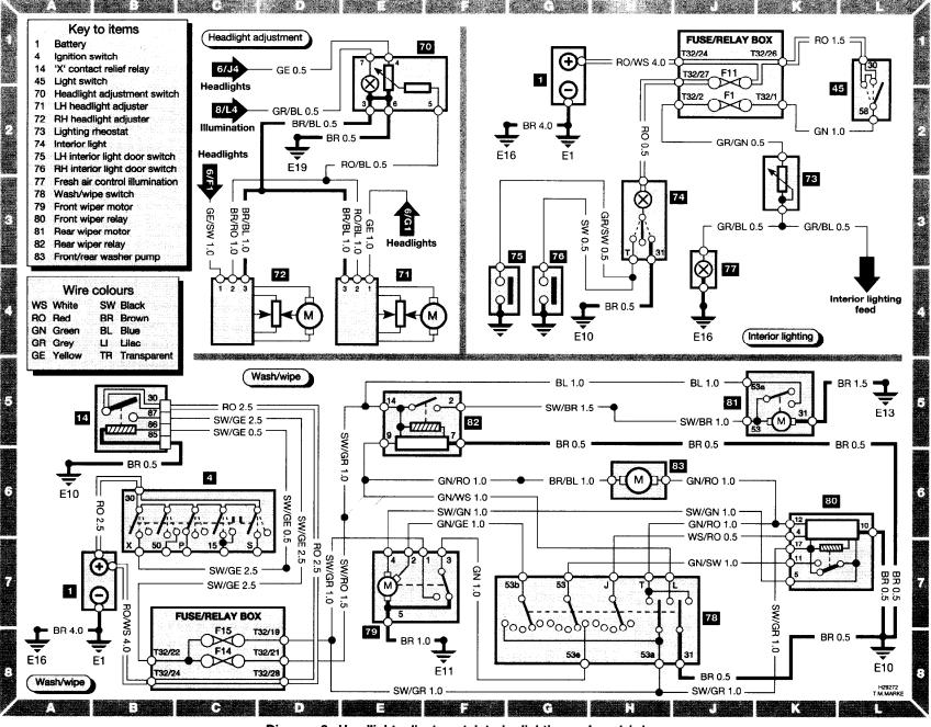
Diagram 8 : Headlight adjustment, interior lighting and wash/wipe
