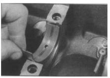
**Bearing** The curved surface on a shaft or in a bore, or the part assembled into either, that permits relative motion between them with minimum wear and friction.
