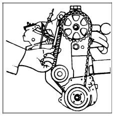
4.15 Testing the timing belt tension
