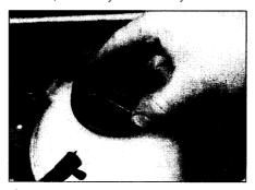
If topping up is necessary, wait until the engine is cold. Slowly unscrew the expansion tank cap, to release any pressure present in the cooling system, and remove it.
