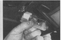
6.3 Remove the festoon type bulb from the contacts
