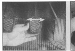
0 Check that the brake pedal is secure and in good condition. Check also for signs of fluid leaks on the pedal, floor or carpets, which would indicate failed seals in the brake master cylinder.
