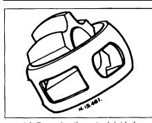
4.8 Removing the outer joint hub from the cage
