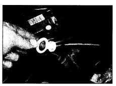
The dipstick top is often brightly coloured for easy identification (see "Underbonnet check points" on page 0.10 for exact location). Withdraw the dipstick from its tube.
