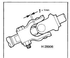
14.9 On later models make sure that the clearance shown is maintained between the end of the steering gear pinion and the universal joint
