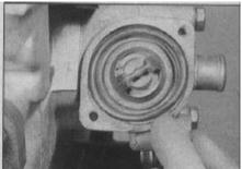
4.3 Removing the thermostat cover sealing ring
