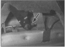
14.5 Handbrake adjusting nut (arrowed)
