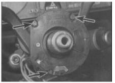
4.4a Steering column combination switch retaining screws
