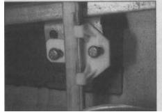
15.3b Bolts securing the lifting plate to the window channel
