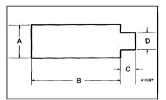
4.13 Clutch driven plate centralising tool dimensions A 18.24 mm B 70.0mm C 20.0mm D 14.81 mm
