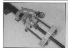
15.1 Draw the splined adapter off the steering column using a puller
