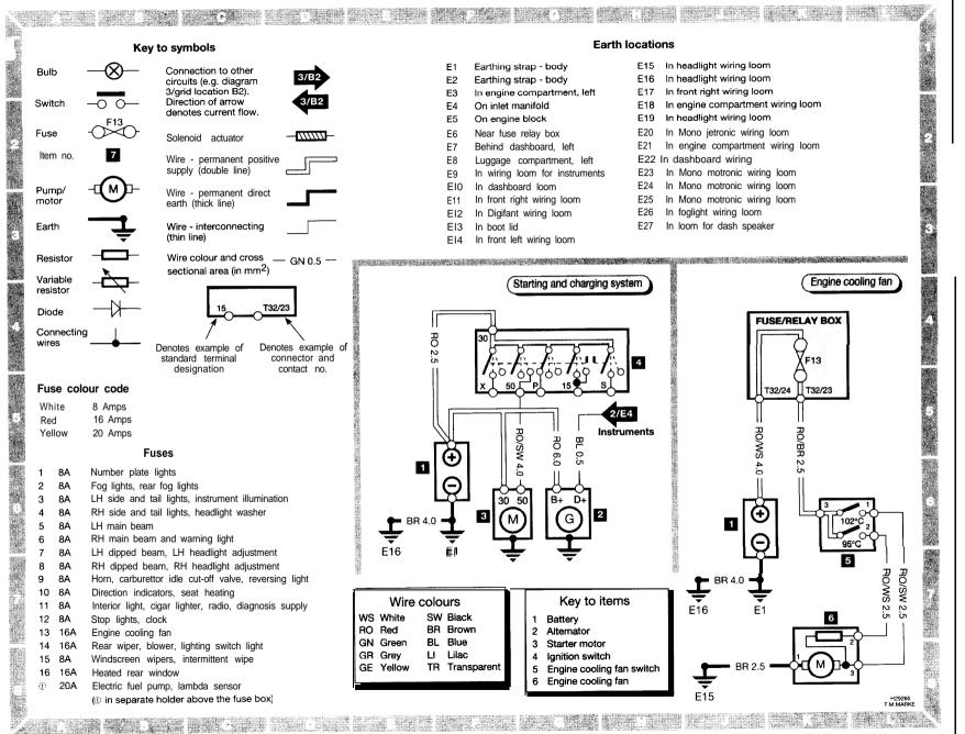
Diagram 1: Information for wiring diagrams, starting, charging and engine cooling fan
