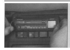
16.3a Fitting the special radio removal tools
