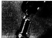
16.9 Adjusting the spark plug electrode gap
