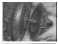
4.15 Fitting the pressure plate assembly
