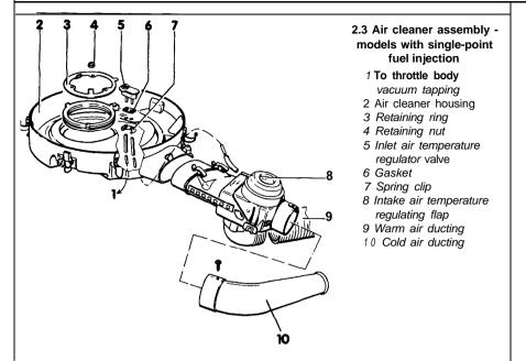
**illustration** 2.3) and remove the temperature regulator from the air cleaner housing. Recover the gasket.
