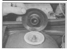
2.10a Removing the front suspension strut top cap
