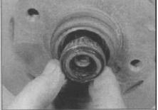
10.4b Removing the rear wheel outer bearing
