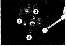
7 Securely tighten the wheel bolts in the sequence shown, Refit the wheel trim, and stow the punctured wheel and tools.
