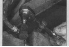
4.4b Removing the caliper mounting bolts
