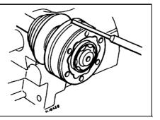
3.13 Removing the plastic cap from the inner joint housing
