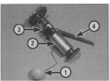
7.12 Fuel pump/gauge sender unit 1 Float and arm 2 Fuel pump 3 Sender unit track and wiper 4 Fuel return hose
