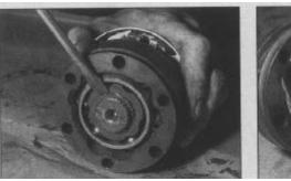
4.16 Removing the inner joint hub and cage
