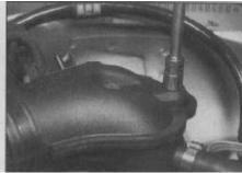
5.24b Remove the bolts, lift off the throttle body inlet elbow . , .
