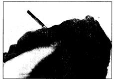
Using a clean rag, remove all oil from the dipstick. Insert the clean dipstick into the tube as far as it will go, then withdraw it again. Keep the handle up so the oil doesn't run along the dipstick to give a false reading.
