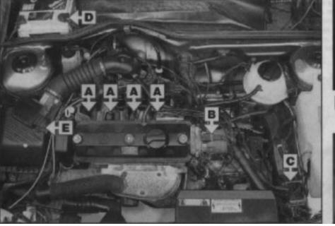
With the ignition switched off, check that electrical connections are secure and spray them with a water dispersant spray, such as **WD40**, if you suspect that moisture may be causing a problem.
