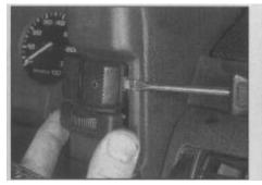
4.7a Using a screwdriver to prise out the lighting switch
