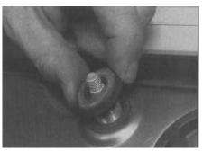
13.2b . . . and remove the spacer
