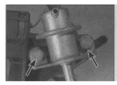
5.45 Remove the retaining screws (arrowed) and lift off the regulator body
