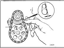
14.17 Checking the oil pump drive chain tension
