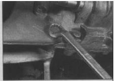
2.14b Removing the rear mounting bracket bolts
