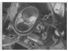
5.28 Slacken and withdraw the four throttle body retaining bolts (three arrowed, one hidden)
