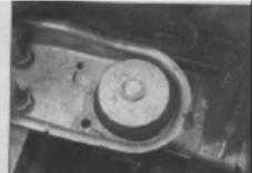
2.20 Front engine mounting through-bolt
