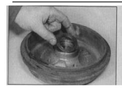
10.11 Grease the lips of the seal, and press it into the rear of the hub
