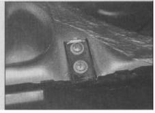
24.12 Screws securing the split rear seat backrest to the luggage compartment floor
