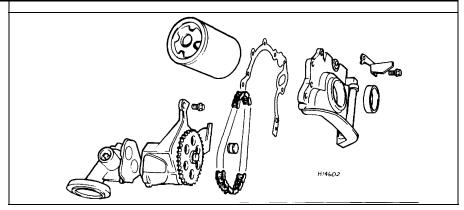
14.1 Exploded view of the oil pump assembly
