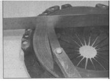
4.8 Checking the clutch pressure plate for taper
