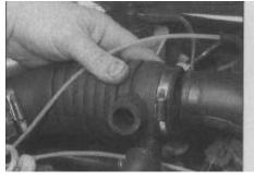
5.24a Slacken the clips and detach the inlet air ducting from the top of the throttle body inlet
