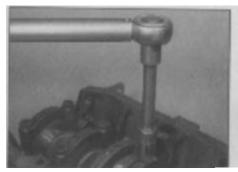
10.18 Tightening the main bearing bolts
