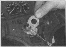
13.3b . . . and remove the washer
