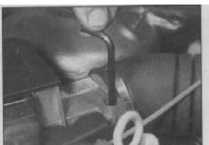
10.3b Exhaust CO adjustment screw location
