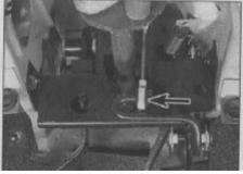
4.5 Unclip the accelerator cable inner (arrowed) from the pedal extension lever
