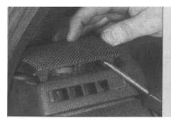
17.1 Use a screwdriver to carefully prise the loudspeaker grille from the facia panel
