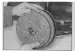
**10** Examine the inside of the drum. Light scoring of the friction surface is normal, but if heavy scoring is found, the drum must be renewed. It is usual to find a lip on the drum's inboard edge which consists of a mixture of rust and brake dust; this should be scraped away.
