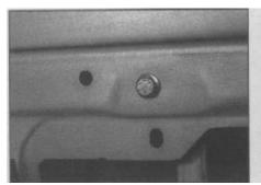
15.6 Bolt securing the front window channel
