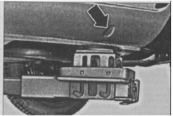
Workshop hoist/trolley jacking point for the rear of the vehicle
