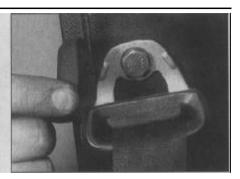
25.7 Removing the plastic cover from the front seat belt upper mounting
