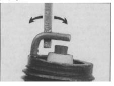
Adjusting spark plug gap
