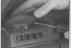
17.2a Depress the tabs to release the loudspeaker from the facia
