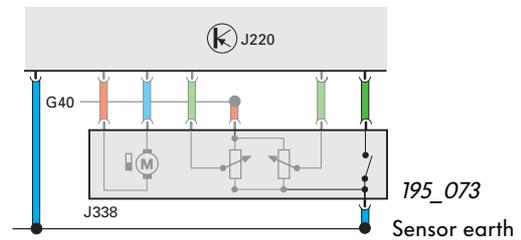
The idling switch utilises the sensor earth of the engine control unit.
