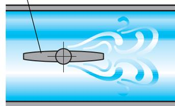
Turbulence during valve control
