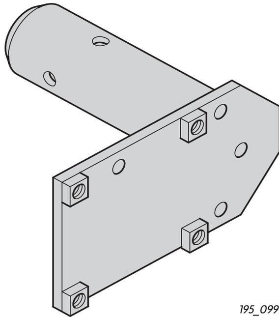
For Counter-holder 3406, position the drill-holes in parallel with the existing drill-hole.
