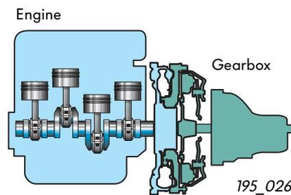
Oscillations produced by the engine █
