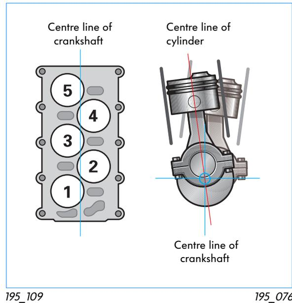
To avoid these overlaps, it was necessary to shift the cylinders slightly further outwards so as to increase the clearance between the cylinders. This process is known as “offsetting”. In the V5 engine the offset of each bank of cylinders is 12.5 mm.
