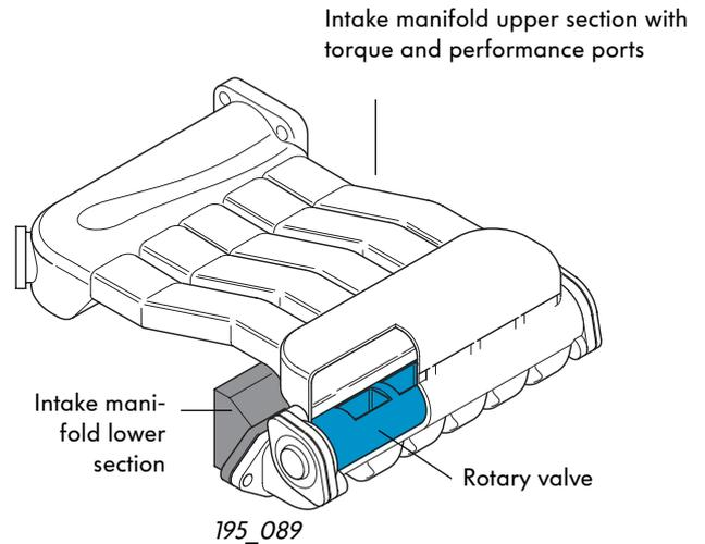
The intake manifold of the V5 engine is based on the ram pipe charge principle.
