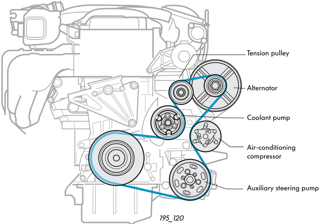
In the transversely mounted engine the coolant pump is integrated in the cylinder crankcase.
