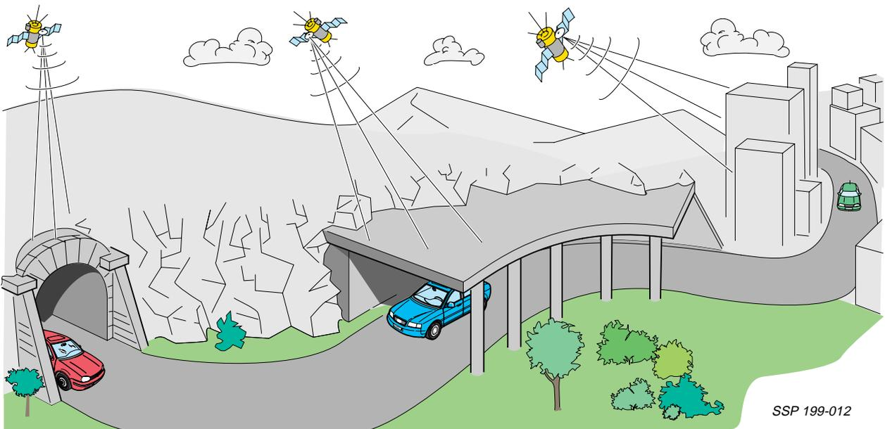
Although the Global Positioning System is the primary source of information for the Radio Navigation System, the system is able to make allowance for short periods of reception interference.
