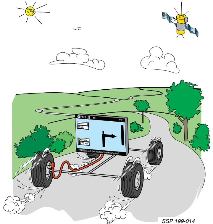
**Vehicle navigation is the overall result of the interplay between satellite navigation and dead-reckoning navigation.**
