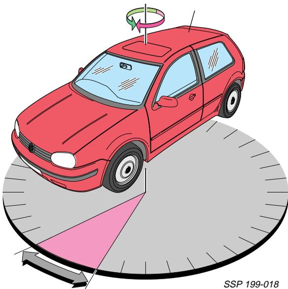
When the vehicle changes its direction of travel, it rotates about its vertical axis.
