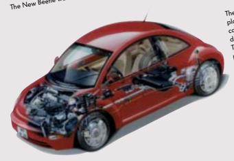
The decision in favour of the Group platform meant that a rear engine could not be used. The engine and drive train are located at the front. The running gear also consists of platform components with a proven track record.
