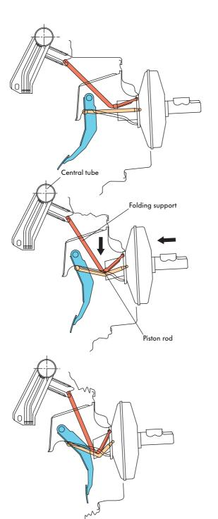
This function is defined by the deformation of the engine bulkhead and does not depend on the position of the brake pedal.
