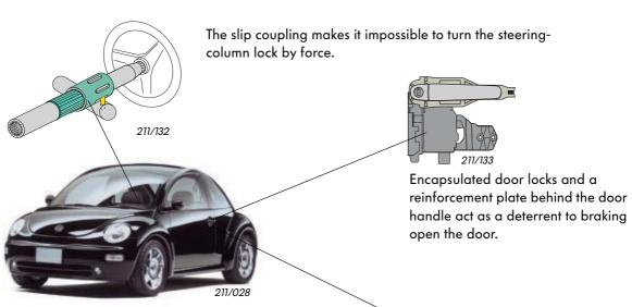
A lock cylinder freewheel is built into the door locks, Boot lock and ignition lock.
