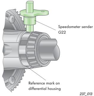
The sender operates according to the Hall sender principle. The electrical impulses generated by the sender are transmited to the control unit in the dash panel insert. Here, the signals are conditioned for the actual road speed and mileage display.
