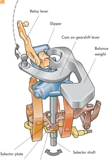
The forward or reverse movement of the gear selector cable during the gearshift causes the selector shaft to rotate.
