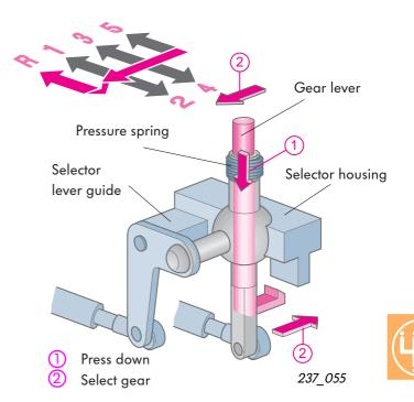
During a normal selection stroke of the forward gears, the locking cam of the gear lever comes up against the lock (an integral part of the selector housing).
