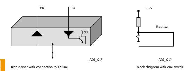
A special feature is the connection of the TX line to the bus. It is normally connected via an open collector.
