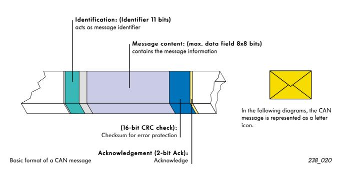
The components of an engine message would therefore include: identifier=engine\_1, content= rpm. The engine message also contains other values, e.g. idling speed, torque etc. The CAN module then checks via the RX line whether the bus is active (whether information is in the process of being exchanged). If necessary, it waits until the bus is free. (Level 1 (passive) for a specific period). If the bus is free, the engine message is sent.
