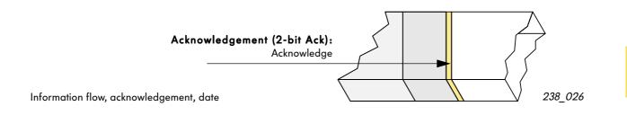
Finally the correctly received message goes to the acceptance section of the associated CAN modules.
