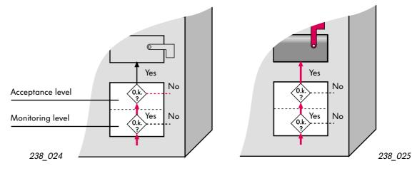
Detail: receive area, monitoring and acceptance levels
