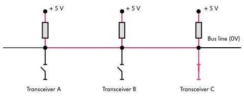
Connection of 3 transceivers to bus line (principle), transceiver C active
