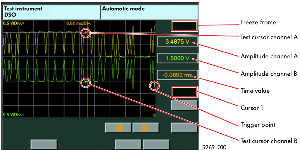
The test cursor should be positioned in the middle of one of the flat impulses to achieve reliable test figures. The displayed measurement shows a drivetrain CAN data bus that has just reached the specified value.
