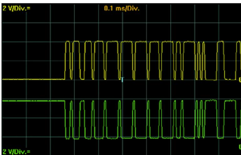
For reasons of clarity, the CAN high and CAN low signal are pulled apart.
