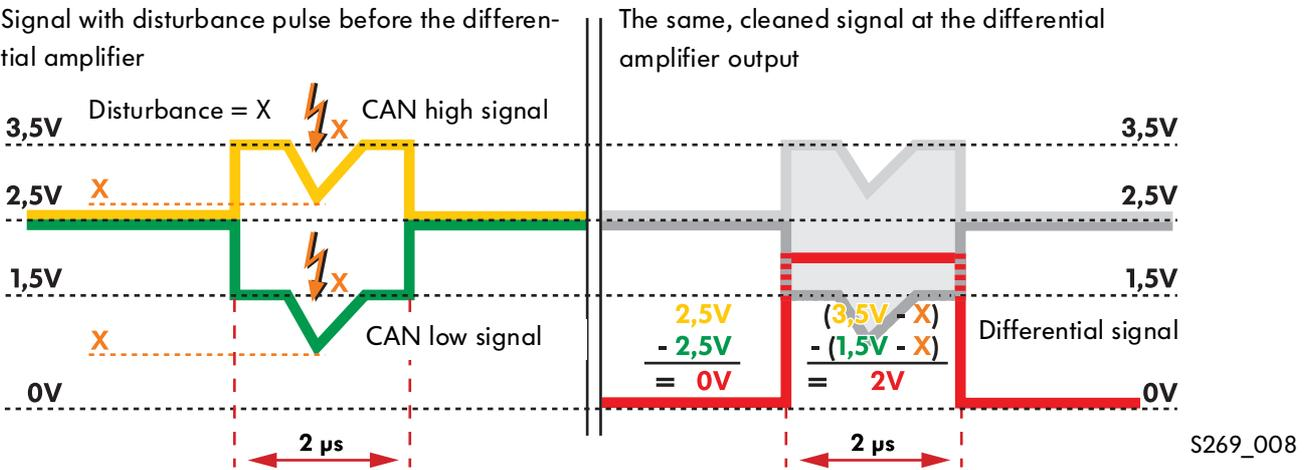
Evaluation of the signals from CAN high and CAN low in the differential amplifier, otherwise known as differential transfer technology, means that the effects of disturbances are practically eliminated. Another advantage of differential transfer technology is the fact that fluctuations in the onboard supply (e.g. when the engine is started) do not affect the transfer of data to individual control units (transfer security).
