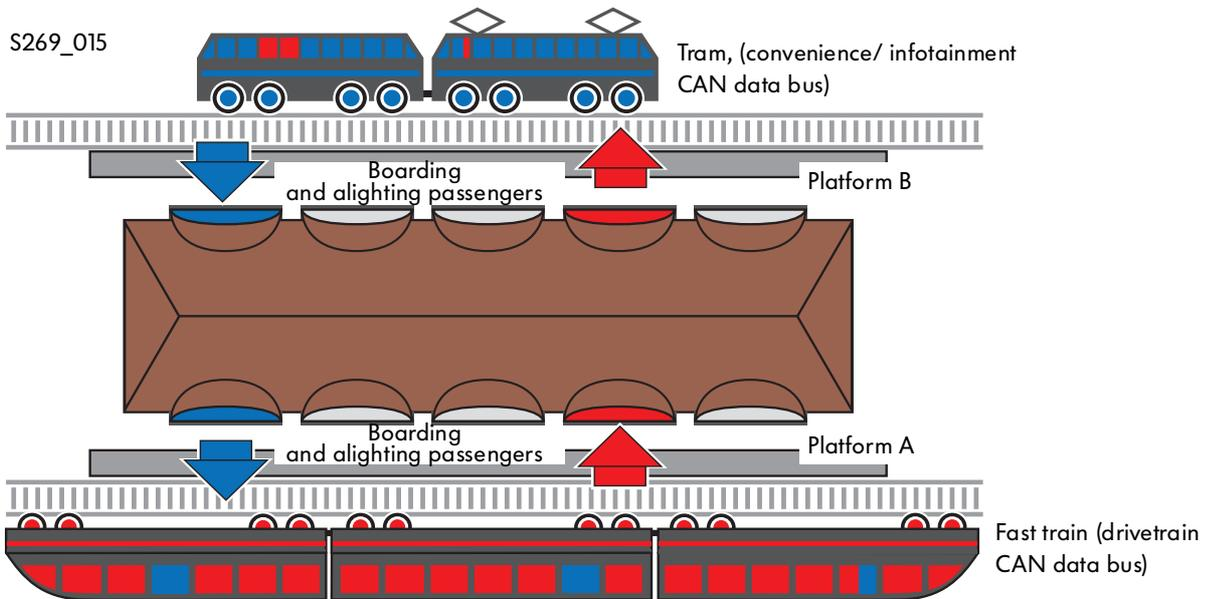
At platform A (otherwise known as the Gateway) of the railway, a fast train arrives (drivetrain CAN data bus, 500 kBit/s) with several hundred passengers onboard.
