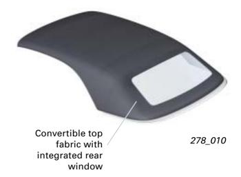
The fabric is mechanically attached by means of fastening strips and sections to the front end of the convertible top, as well as to roof frame, bracing hoops and convertible top frame.
