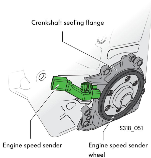
The engine speed sender wheel consists of a steel ring coated with a rubber compound. This rubber compound contains a large number of metal chips which are alternately magnetised to become north and south pole regions. The diesel engines have two large north poles (60-2-2) and the petrol engines have one large north pole (60-2) on the sender wheel; they serve as reference marks for the engine speed sender. The sender wheel is press-fitted onto the crankshaft flange and exactly positioned.
