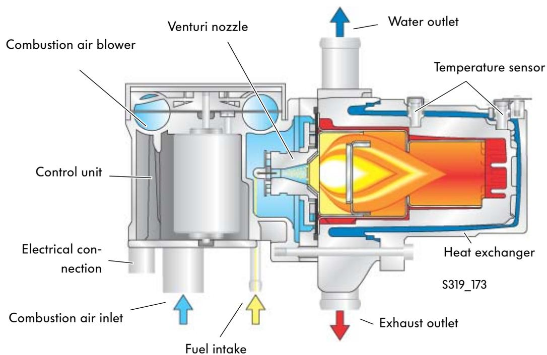
The Intake air is ducted through a ceramic housing which is shaped to form a Venturi nozzle. Fuel injection is assisted by the suction effect.
