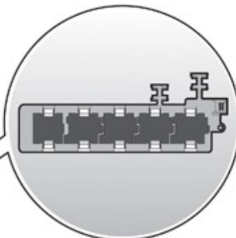
Relay carrier below the dash panel on the left, above the onboard power supply control unit
