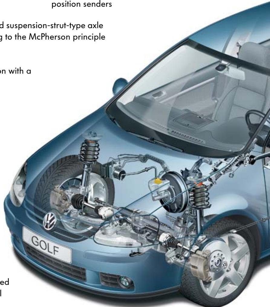
The Golf can be equipped with a standard running gear, sports running gear or heavy-duty running gear. The running gear packages are distinguished in terms of their springs, dampers, anti-roll bars and the bearing elements. The sports running gear has been lowered 15 mm compared to the responsive and yet comfort-oriented standard running gear. The heavy-duty running gear has been lifted 20 mm compared to the standard running gear.
