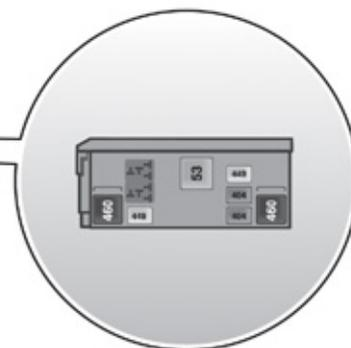
Relay carrier in the onboard power supply control unit, below the dash panel on the left
