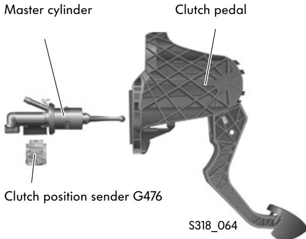
The clutch position sender is a Hall sensor, which signals to the engine control unit that the clutch pedal has been operated. The cruise control system will then be deactivated and the injection quantity in the engines will briefly be reduced in order to prevent engine shudder during the gear change.
