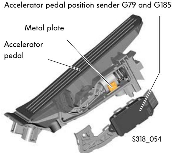
The two accelerator position senders G79 and G185 are integrated in the upright accelerator pedal module. They are inductive senders, which indicate the exact position of the accelerator pedal the engine control unit. From this data, the engine control unit computes the required injection quantity.
