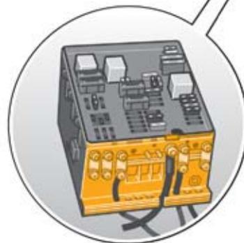
Back-up fuse box in the engine compartment on the left
