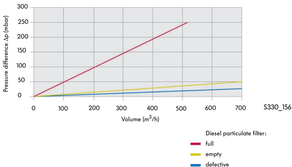
The engine control unit creates a ratio from the pressure difference and the volume of exhaust gas and can thus calculate the flow resistance of the particulate filter. From the flow resistance, the engine control unit can detect the level of carbon deposit.
