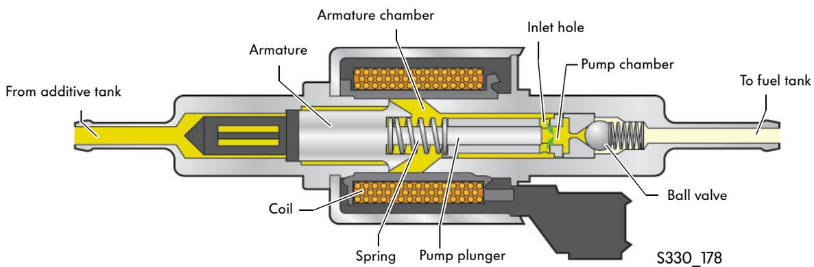
The pump plunger moves to the start position. The vacuum generated as a result draws additive in through the open inlet hole from the armature chamber to the pump chamber.
