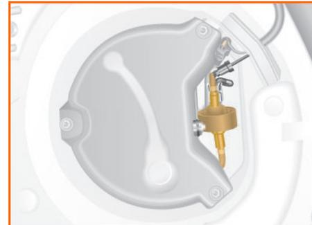
The particulate filter additive pump is of the reciprocating piston type, which delivers additive to the fuel tank. It can be found bolted on the additive tank.
