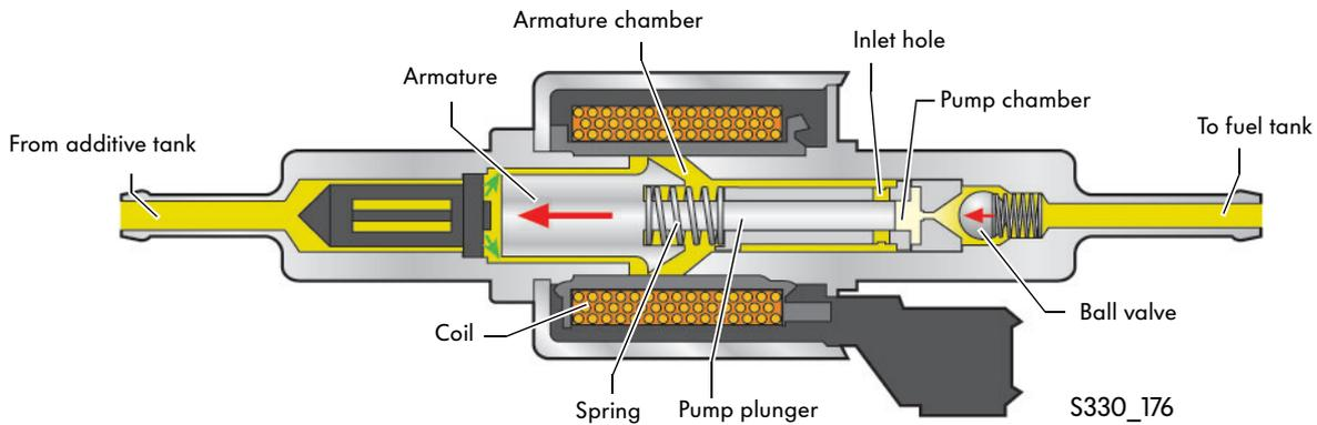
During intake, the additive flows into the armature chamber. The magnetic coil is not actuated by the engine control unit and the spring presses the pump plunger back. At the same time, the ball valve closes the pump chamber.
