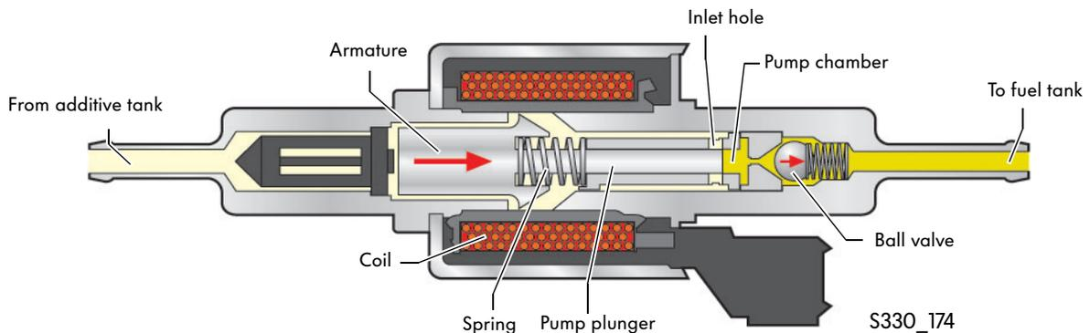
When not energised, the pump is filled with additive. As soon as the engine control unit actuates the particulate filter additive pump, the coil is energised and the armature moves the pump plunger against spring pressure. The pump plunger closes the inlet hole to the pump chamber and forces the additive in the chamber towards the ball valve.
