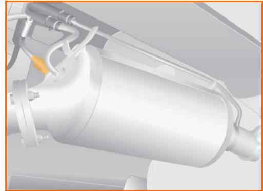
The temperature sender before particulate filter is a PTC sensor. On a sensor with PTC (positive temperature coefficient), resistance rises as temperature increases.
