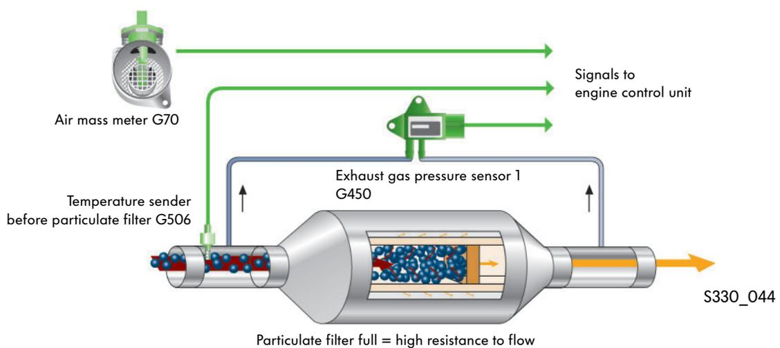
During regeneration, the tiny particles of carbon stored in the particulate filter are burnt off. This occurs every 500-700 kilometres, depending on the way the vehicle is driven, and lasts about 5-10 minutes. There are no signs to the driver that regeneration is occurring.
