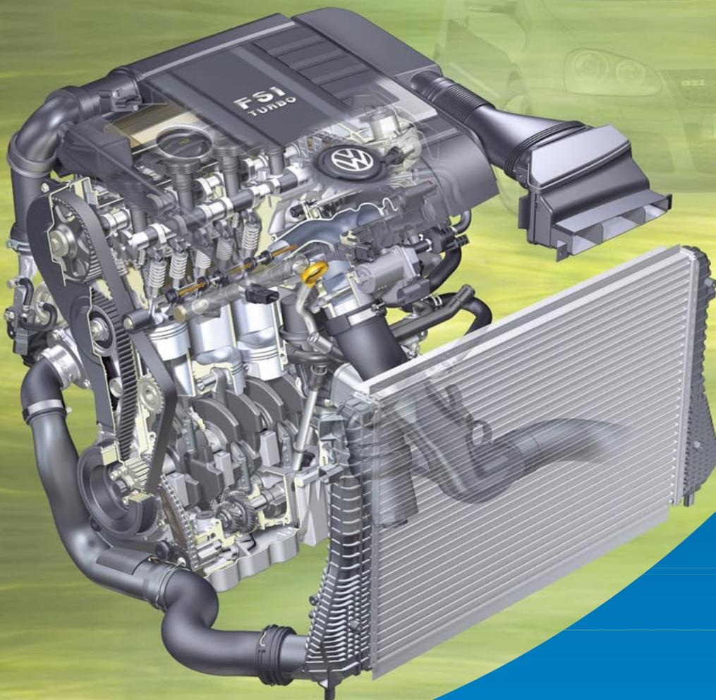
The new FSI engines from Volkswagen do without stratified injection and place greater emphasis on output and torque. Until now, FSI direct injection was always associated with stratification. On the turbocharged engine, the abbreviation FSI remains but there is no stratified charge. Doing without fuel stratification and NOx sensors represents a loss on one part, but also promises the finest driving enjoyment with high output and a torquey engine and great pulling power and economy.
