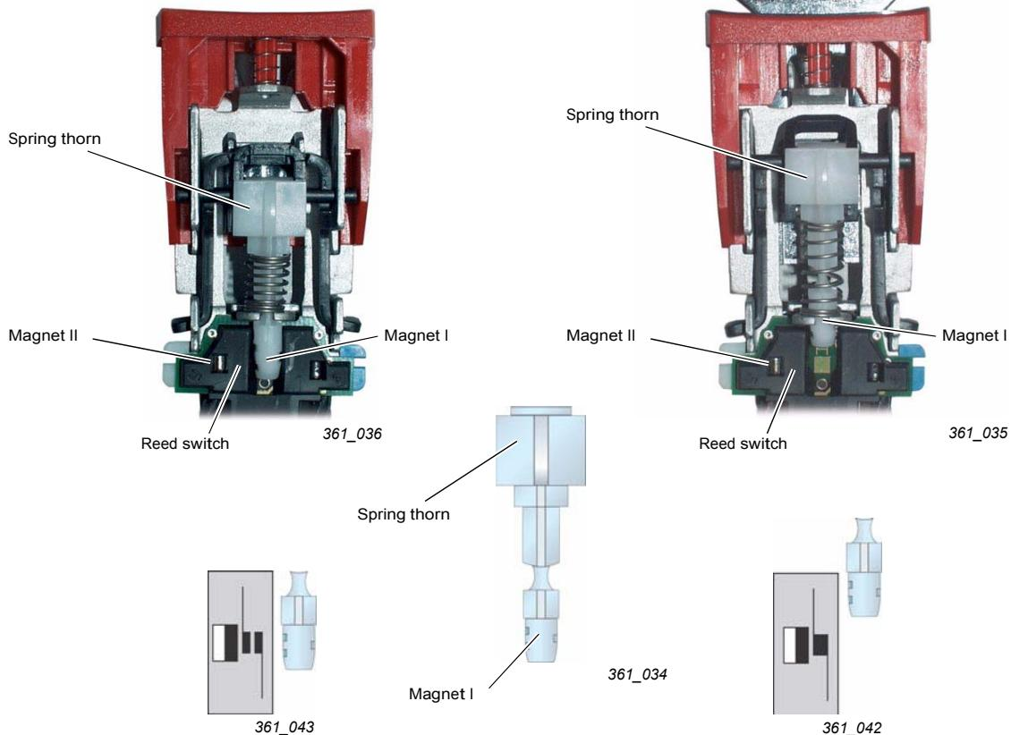
Two resistors are integrated in the circuit. Depending on the position of the reed switch, measurement takes place via one or both resistors. Based on the measured resistance value, the airbag control unit recognises whether the seat belt is fastened or not.
