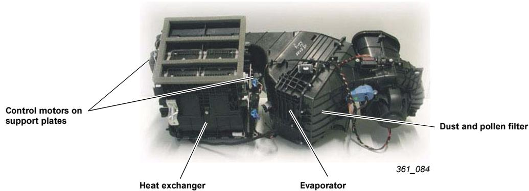
Most of the control motors can be replaced with the dash panel in place; the specific repair operations are described in the Workshop Manual.
