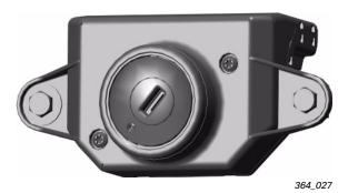
• Evaluating the key position in the ignition switch with 4 microswitches
