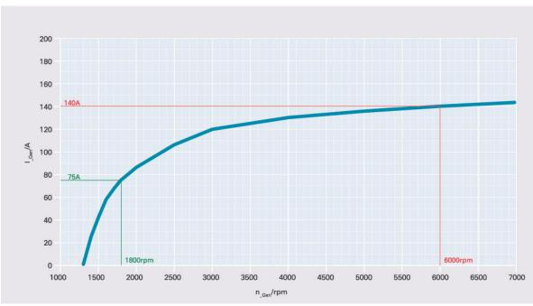
Close attention is normally given to two operating points. This is firstly the point at 1800 rpm (equivalent to idling speed, green marks) and, secondly, the setpoint at 6000 rpm (red mark). In the case of an 140 A alternator, for example, this value always refers to the setpoint at 6000 rpm. Some nameplates display values such as 75-140 A. The first value denotes the maximum possible current output at 1800 rpm, i.e. 75 A, and the second value corresponds to the setpoint (140 A at 6000 rpm).
