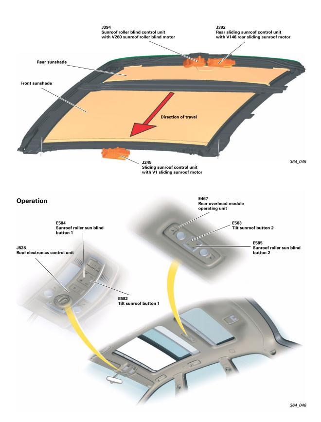
Glass section 1 can be operated using the rotary switch for the sliding sunroof in the front overhead module. Glass section 3 can be operated using the tilt sunroof button 1 E582 in the front overhead module and tilt sunroof button 2 E583 in the rear overhead module operating unit E467. Automatic opening/closing mode is activated by briefly pressing the button. Manual opening/closing mode is activated by holding the button down.
