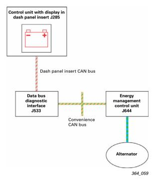
The alternator or the regulator in the alternator can send 3 fault messages via the bit-synchronous interface to the energy management control unit:
