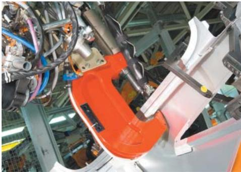
Solid punch riveting process in production
