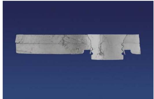
Micrograph of a solid punch riveted joint
