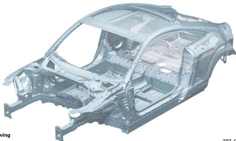
Applications of Flow Drill screwing
