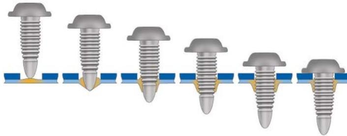
Flow Drill screwing process
